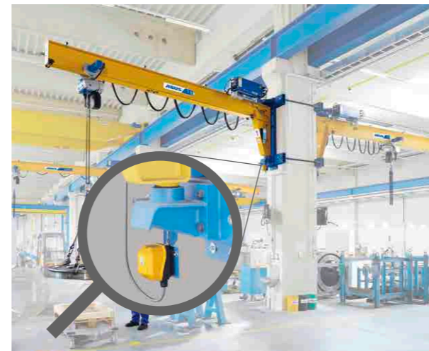
Slewing limit switch, VW (Fig. 7)
