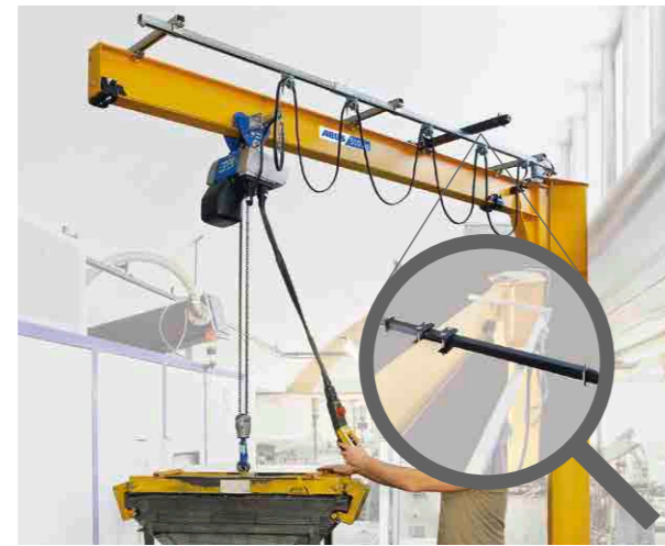
Slewing limit stop – bumper rod (Fig. 4)
