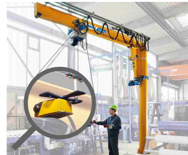
Limit switch for trolley travel (Fig. 8)
