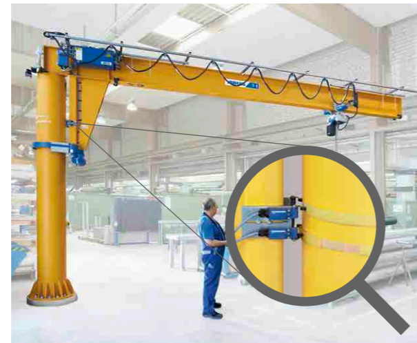
Slewing limit switch, VS (Fig. 6)
