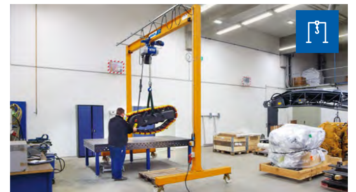
Lightweight mobile gantry LPK
